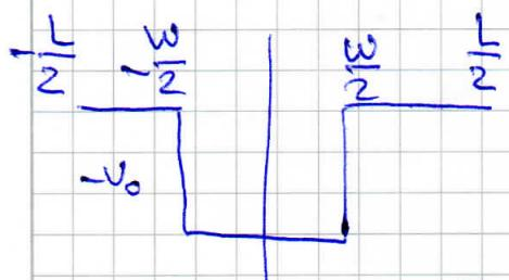
$$\tilde{V}(G) = \frac{-V_0}{L} \int_{-L/2}^{L/2} dz e^{-iGz} = -\frac{2V_0}{LG} \sin \frac{Gw}{2}$$
