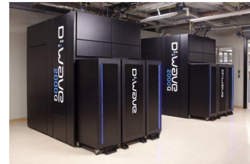
~2000 qubit quantum annealing device (adiabatic computing) (D:WAVE, 2017)
