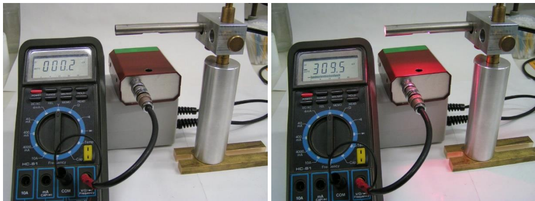
Figure 2. Operating “solar blind” UV photodetector containing an AlGaN layer. The detector illuminated with day light generates 0.2 mV voltage, whereas after illumination using a mercury lamp, the generated voltage is over 300 mV and can be measured with a universal multimeter.
