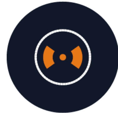
Schematic of the fiber geometry showing the bow-tie configured stress elements and the step index core.
