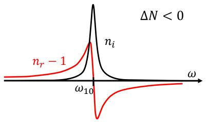
schematic drawings for low pressure atomic gas or low density ions
