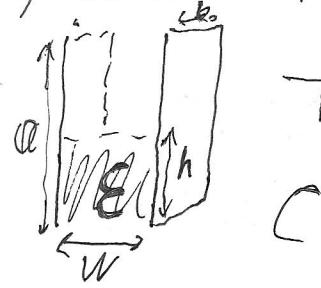
$$\frac{1}{C} = \frac{1}{C_1} + \frac{1}{C_2} \quad C_1 = \frac{\epsilon_0(a-h)}{W}, \quad C_2 = \frac{\epsilon_0 \epsilon h}{W}$$
